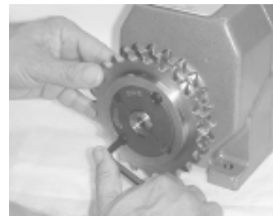
TIGHTEN SCREWS ALTERNATELY
